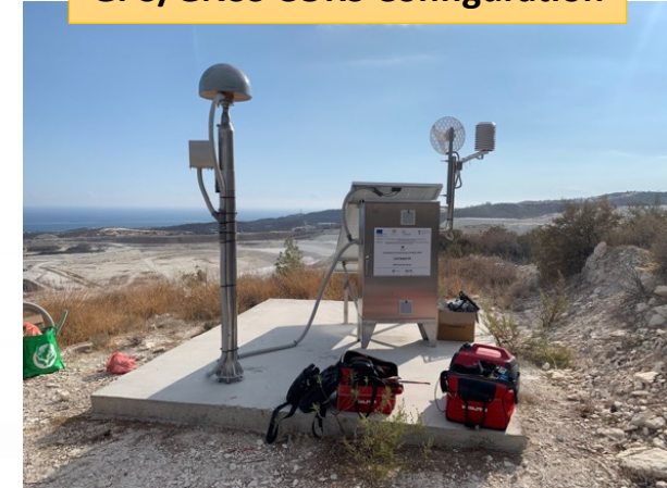
Example of a Mobile GPS/GNSS CORS Configuration
